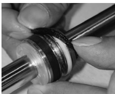
Picture 8: Installation of piston seal
